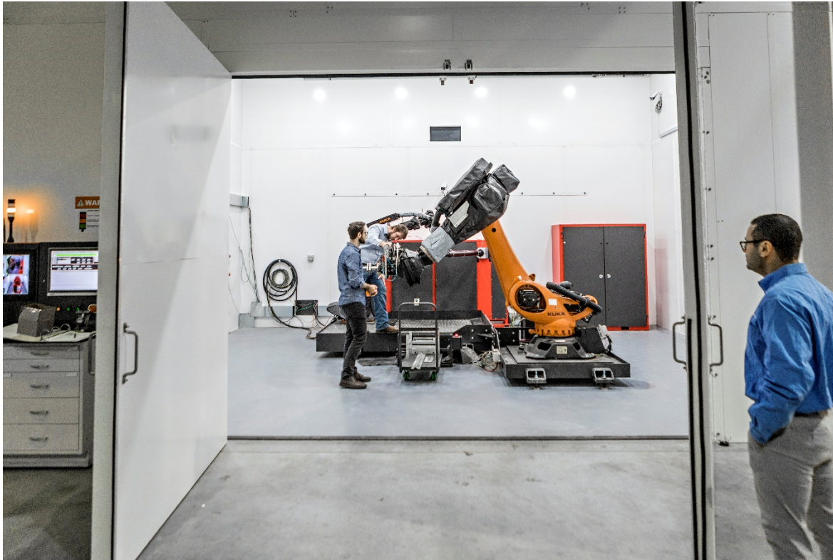
Figure 4. Processing cell for Procudo ® 200 Laser Peening System showing beam delivery tables and the robot for manipulating parts during processing. The laser system is on the other side of the wall behind the cabinets.
