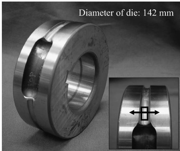
Fig. 1 – A standard pilger die. The location of the residual stress measurement and the orientation of the X-ray are indicated by a circle and a double-headed arrow, respectively in the insert.
