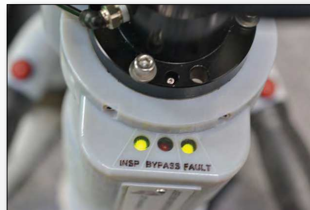
Green lights on the inspection head denote a good bond is present
