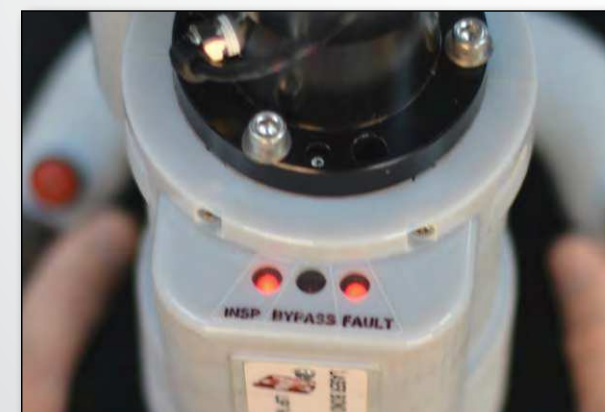
Red lights on the inspection head denote a bad bond is present
