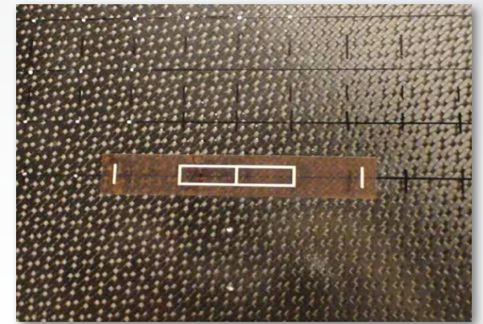
Inspection tape with copper trace for EMAT
